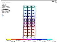
Fig.4.Ten storied building with locked brick infill walls
